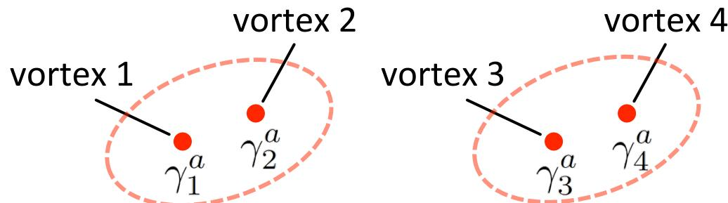
$$\text{Dirac fermion operator} \quad \Psi_1^a = \frac{1}{2} (\gamma_1^a + i\gamma_2^a) \quad \Psi_2^a = \frac{1}{2} (\gamma_3^a + i\gamma_4^a) \quad (\text{Triplet})$$
