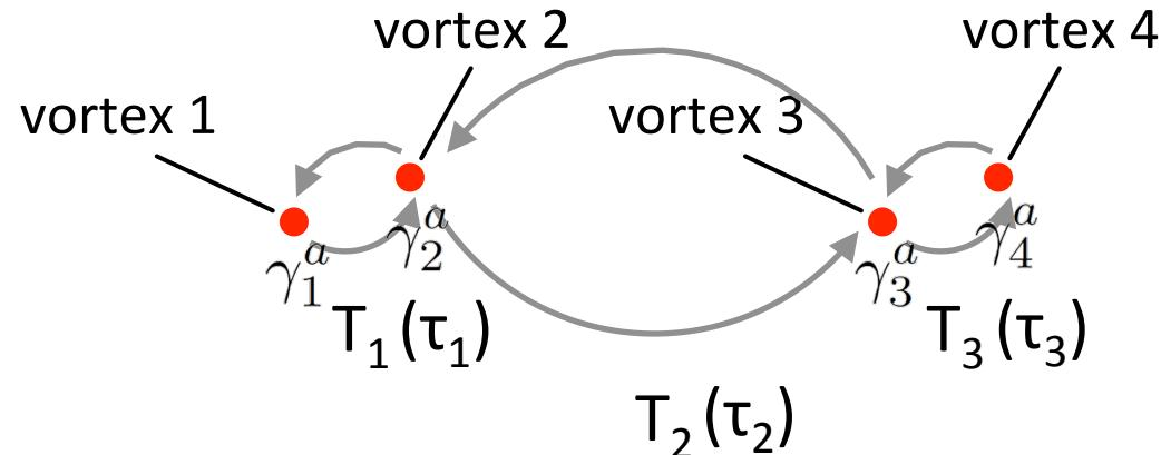
1) Exchange operator :  $\tau_k = \prod_{a=1,2,3} \frac{1}{\sqrt{2}}(1 + \gamma_{k+1}^a \gamma_k^a)$        $\gamma_l^a \rightarrow \tau_k \gamma_l^a \tau_k^{-1}$
