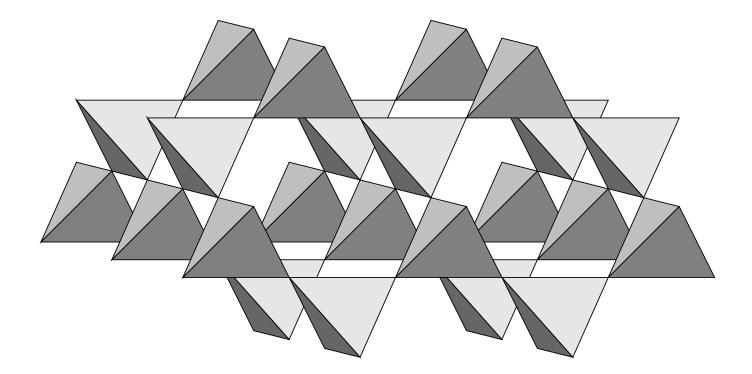
Coordination four lattice of corner linked tetahedra. The rare earth ions occupy the vertices of the tetrahedra; **e.g.**  $Dy_2 Ti_2 O_7$
