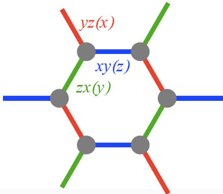
$$H = \sum_{\langle ij \rangle \in \alpha\beta(\gamma)} [JS_i \cdot S_j + KS_i^\gamma S_j^\gamma + \Gamma(S_i^\alpha S_j^\beta + S_i^\beta S_j^\alpha)], \quad (1)$$
