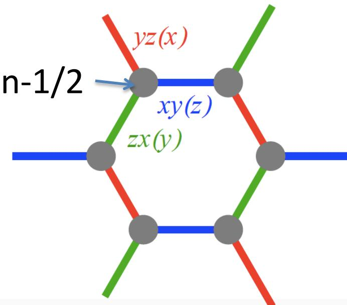
$$H = K_x \sum_{\langle ij \rangle \in \text{yz}(x)} S_i^x S_j^x + K_y \sum_{\langle ij \rangle \in \text{zx}(y)} S_i^y S_j^y + K_z \sum_{\langle ij \rangle \in \text{xy}(z)} S_i^z S_j^z.$$
