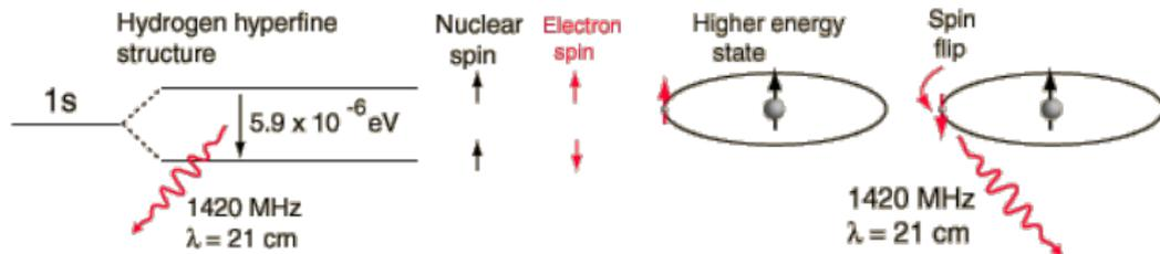
Spin-parallel (higher energy)  $\rightarrow$  spin-antiparallel (lower energy)
