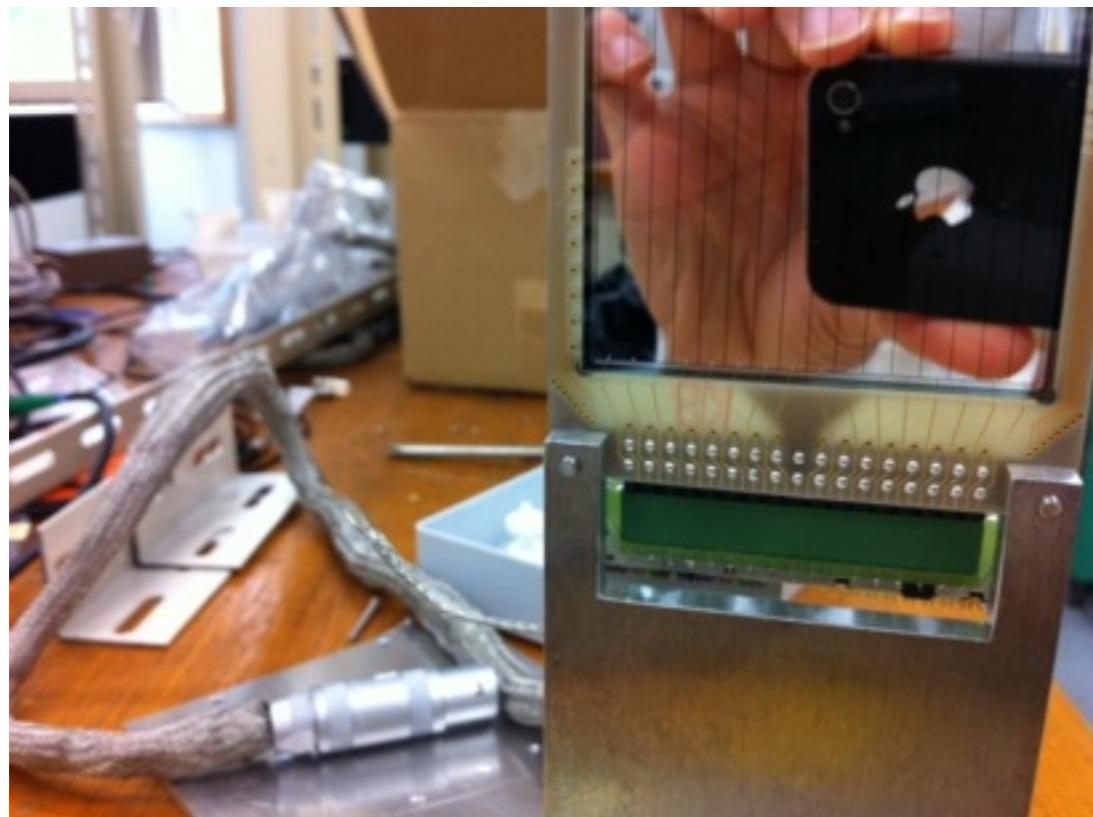
prototype MWDC in construction
