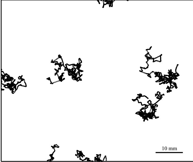
FIGURE 3. Typical trajectories of particles in the horizontal cell under the microgravity (steady state). Seven particles during 1.6sec are picked up and shown. The frequency and the acceleration of external vibration are 100 Hz and 48 \text{ m sec}^{-2} , respectively.
