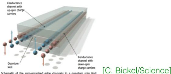
Schematic of the spin-polarized edge channels in a quantum spin Hall insulator.
