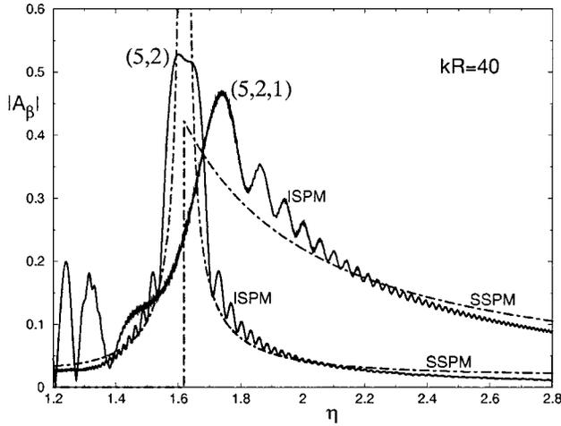
FIG. 1. Moduli of amplitudes  $|A_\beta|$  vs  $\eta$  for the equatorial “star” orbit (5,2) ( $\mathcal{K}=1$ ) and the 3D orbit (5,2,1) ( $\mathcal{K}=2$ ) bifurcating from it at  $\eta=1.618\dots$ . Solid lines: using the ISPM according to Eqs. (9) and (6), respectively; dash-dotted lines: using the standard stationary-phase approach.
