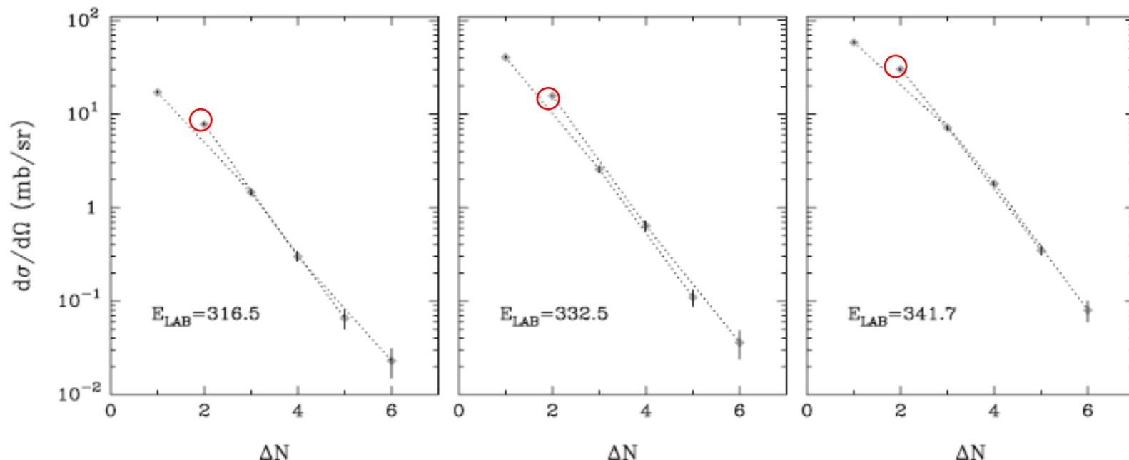
**Figure 38.** Results for the one- to six-neutron transfers from the reaction  $^{62}\text{Ni} + ^{206}\text{Pb}$  at different energies covering overlap parameters up to  $d_0 = 1.4$  fm. The small enhancement of the two-neutron transfer can be seen. The deviation of the higher-order transfers from the exponential fall-off defined by the 1n transfer defines here the enhancement factor EF (see also figures 23 and 46).
