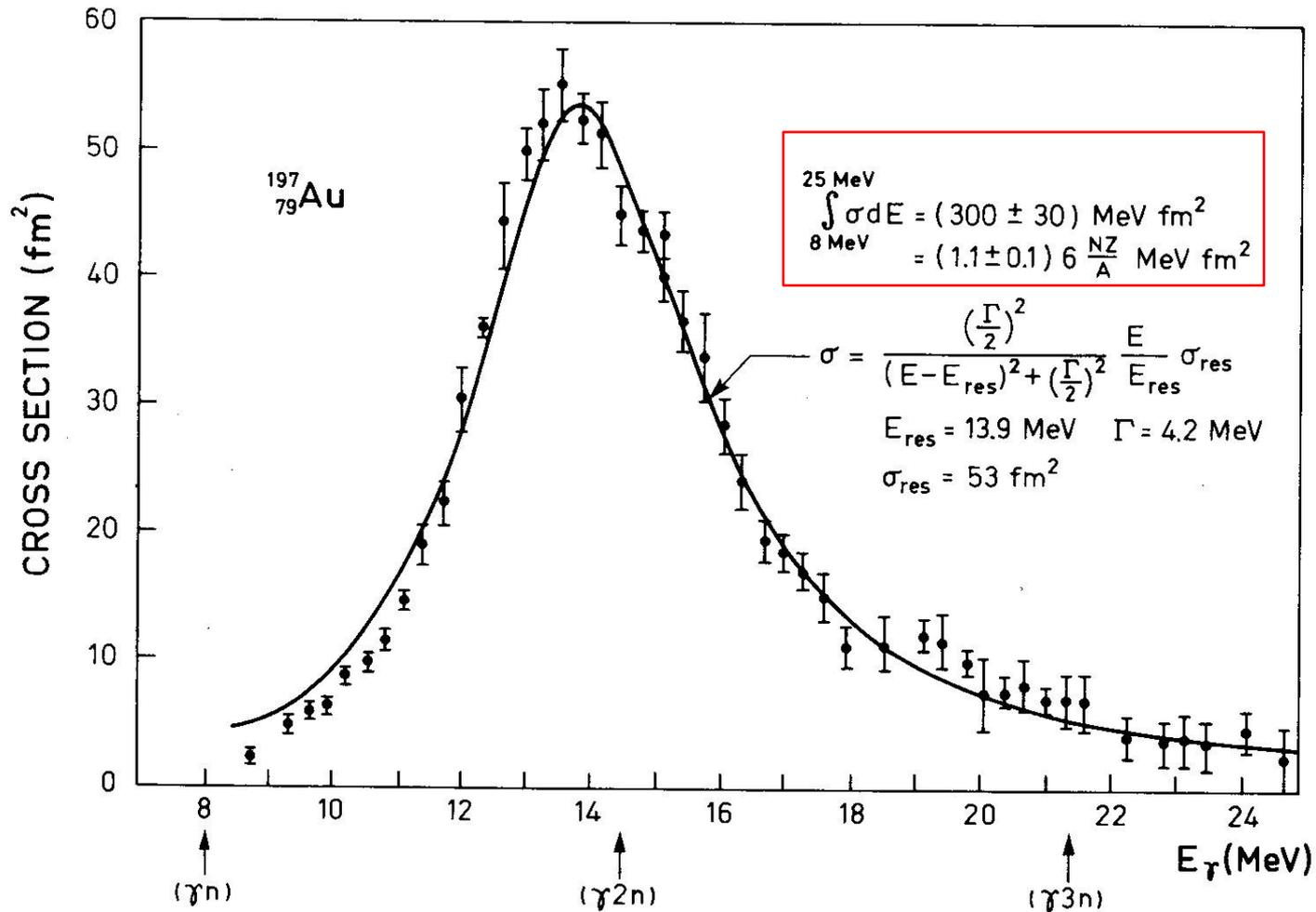
**Figure 6-18** Total photoabsorption cross section for  $^{197}\text{Au}$ . The experimental data are from S. C. Fultz, R. L. Bramblett, J. T. Caldwell, and N. A. Kerr, *Phys. Rev.* **127**, 1273 (1962). The solid curve is of Breit-Wigner shape with the indicated parameters.
