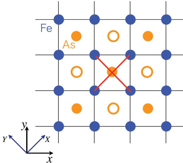
Along a symmetric direction in the momentum space, the degeneracy of the two atomic orbitals  $zx$  and  $yz$  on Fe are lifted.
