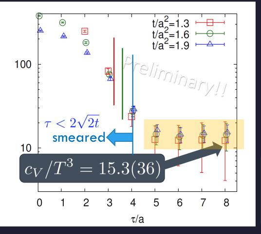
T=2.31Tc b=7.2, Nt=16 2000 confs p=0 correlator specific heat  $\frac{\langle \delta E^2 \rangle}{VT^2}$  $c_V = \rightarrow$  Novel approach to measure specific heat! Gavai, Gupta, Mukherjee, 2005  $c_V/T^3 = 15(1)$   $T/T_c = 2$
