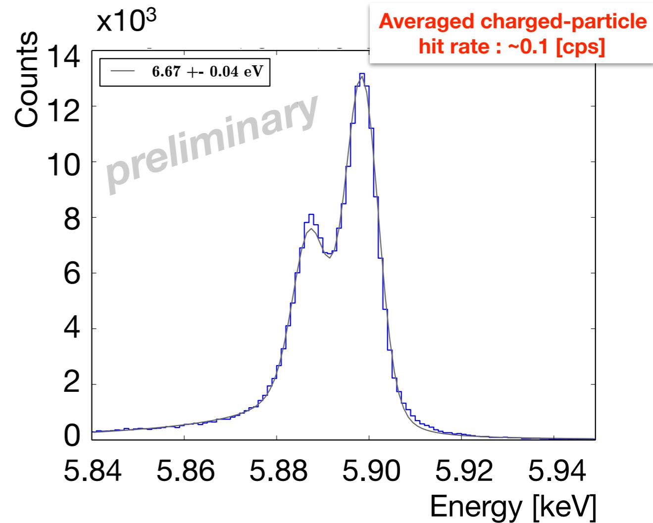
If no lead shield,  $\Delta E > 10 \text{ eV}$ .  $\Rightarrow$  **Lead shield was quite effective.**
