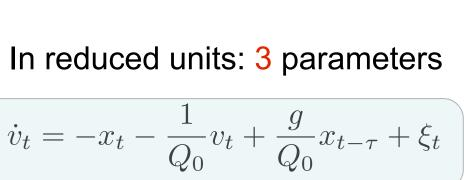
describes accurately the dynamics of nanomechanical resonators (e.g. the cantilever of an AFM) used in feedback cooling setups.
