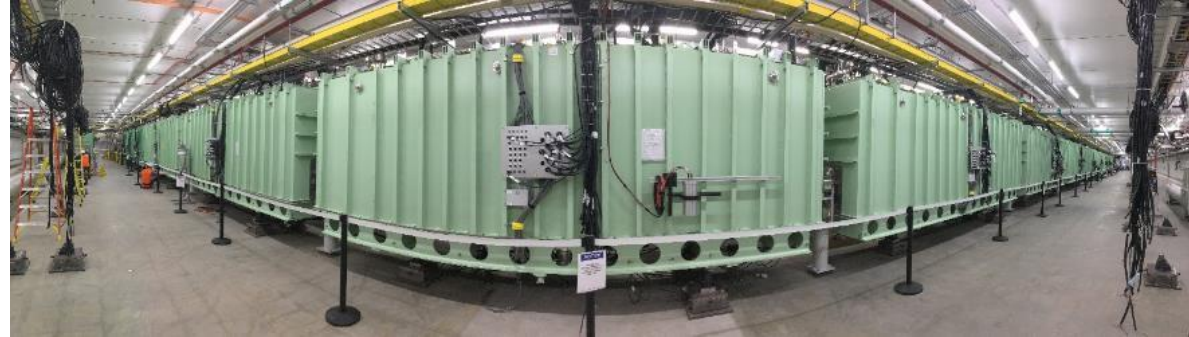
Panoramic view of linear accelerator cryomodules
