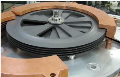
Multi-slice rotating graphite target
