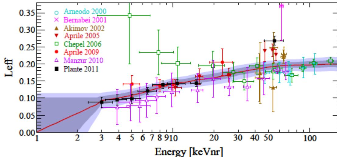
Scintillation efficiency as a function of energy
