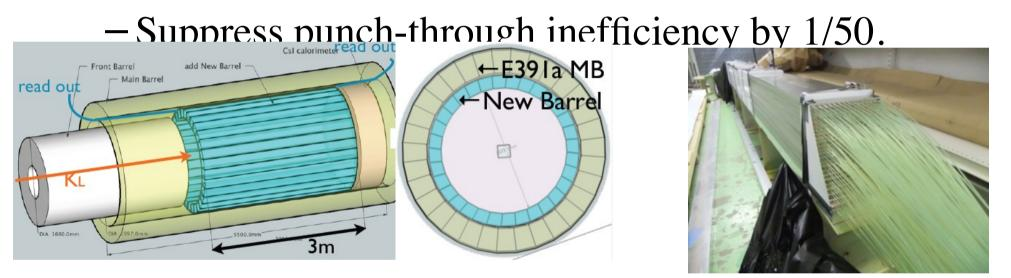
Gluing fiber to scintillator was mostly finished. Module assembly will start soon. Will install it in this winter
