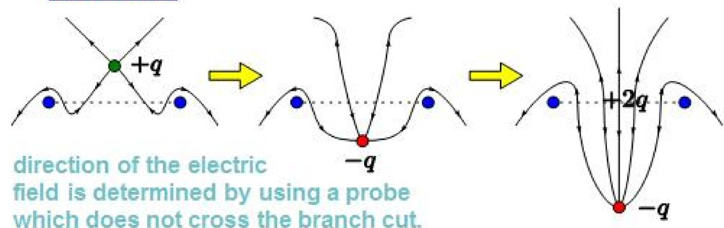
Non-localized charge, called Cheshire charge, appears on the branch cut, and the total charge Is kept invariant under the above process.
