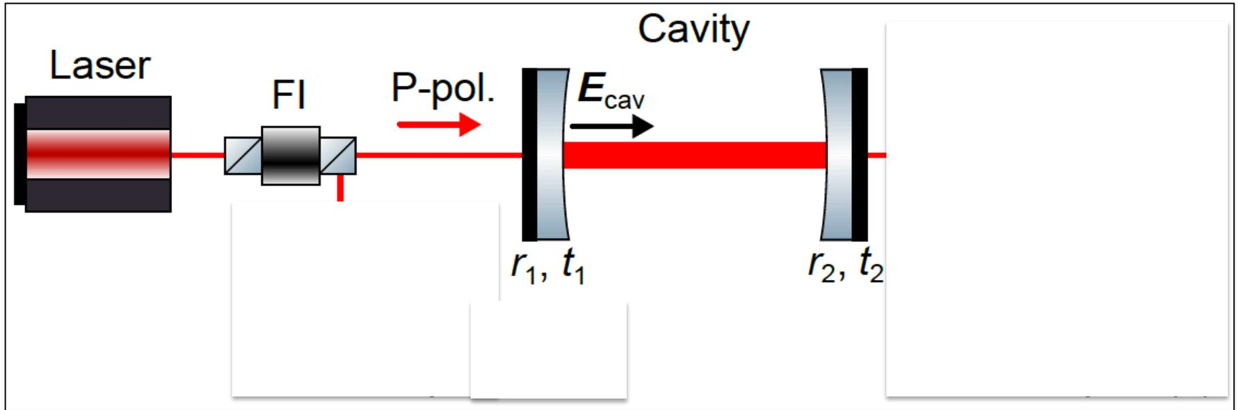
$$\begin{aligned} \mathbf{E}_{cav}(t) &= \frac{t_1 E_0 e^{ikt}}{1 - r_1 r_2} \begin{pmatrix} e^L & e^R \end{pmatrix} \begin{pmatrix} 1 + i\delta\phi(t) & 0 \\ 0 & 1 - i\delta\phi(t) \end{pmatrix} \frac{1}{\sqrt{2}} \begin{pmatrix} 1 \\ 1 \end{pmatrix} \\ &= \frac{t_1}{1 - r_1 r_2} [\mathbf{E}^p(t) - \delta\phi \mathbf{E}^s(t)] \quad (2kL = 2\pi N) \end{aligned}$$
