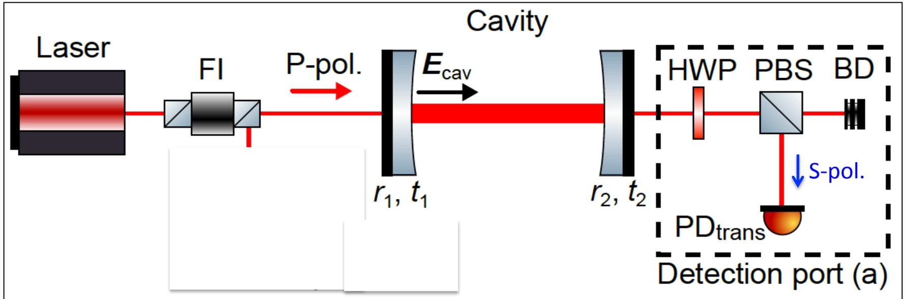
$$E_{PD}(t) = \frac{t_1 t_2}{1 - r_1 r_2} (\alpha - \delta\phi) E^s(t) \quad \alpha \ll 1 : \text{mixing angle}$$
