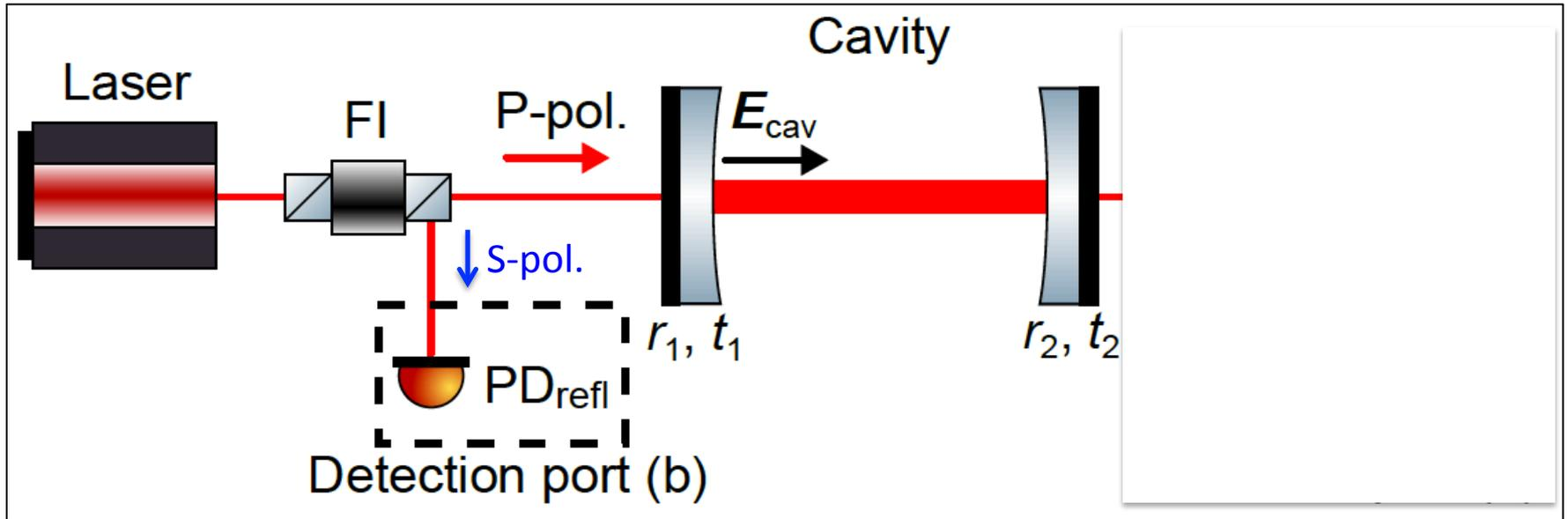
$$E_{PD}(t) = \frac{t_1 t_1}{1 - r_1 r_2} (\alpha - \delta\phi) E^S(t) \quad \alpha \ll 1 : \text{mixing angle}$$
