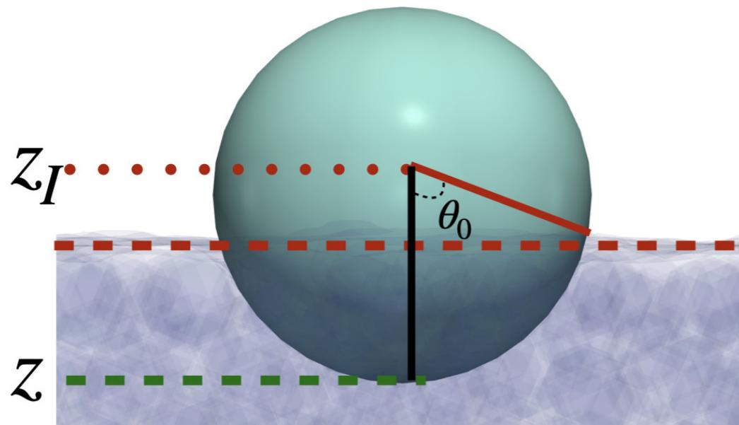
Drag on the impactor is proportional to its depth before completely immersed
