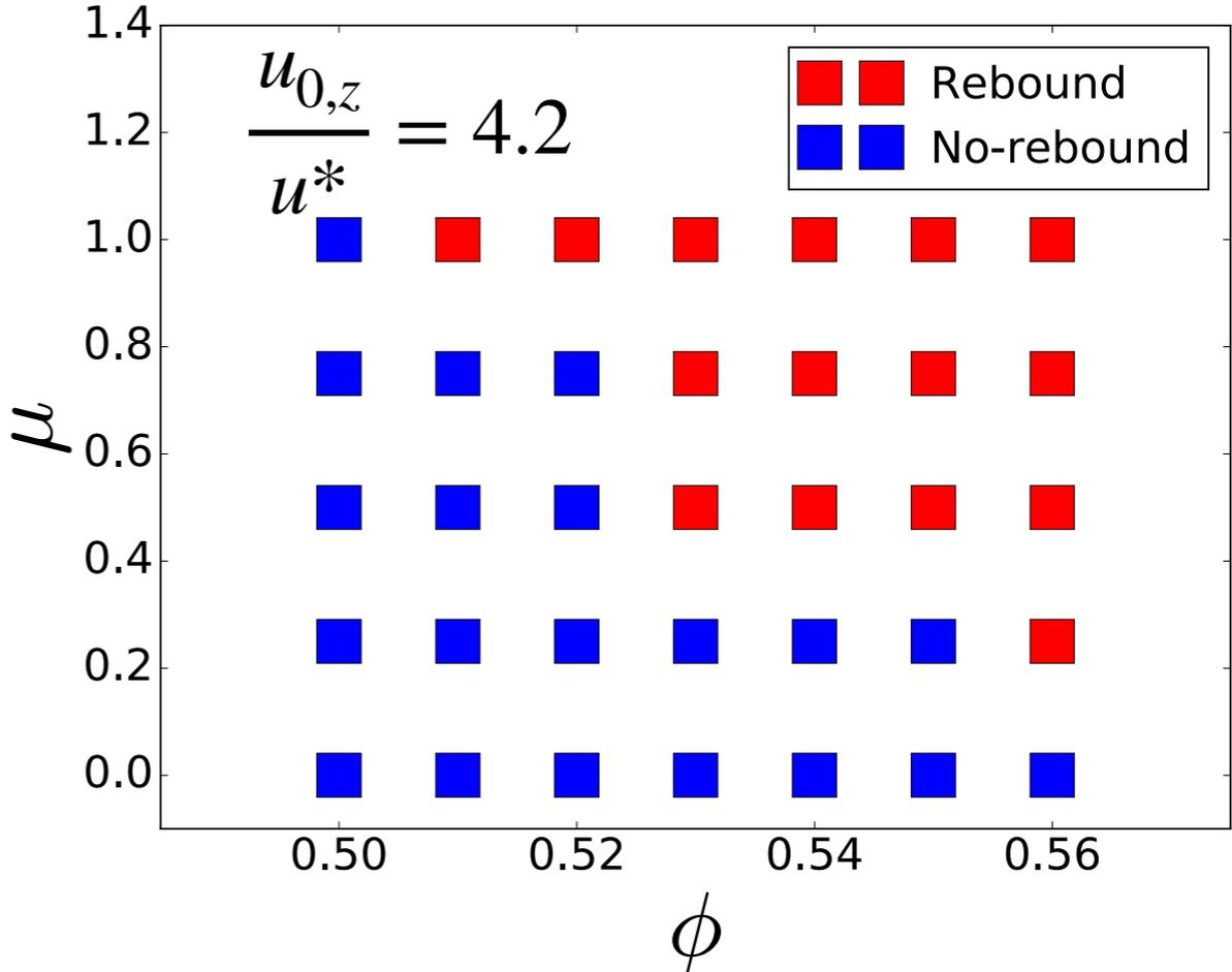
Frictional interaction increases the contact duration between particles that leads to a stronger hardening
