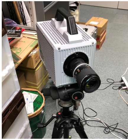
High speed camera (FASTCAM SA1.1) Frame rate = 10000 f sec -1
