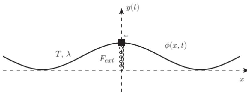
$$S = \int dt \left[ \frac{m}{2} \dot{y}^2 - U_{\text{ext}} \right] + \int dt dx \left[ \frac{\lambda}{2} \dot{\phi}^2 - \frac{T}{2} \phi'^2 \right] - \int dt Q(t) [\phi(x=0) - y]$$
