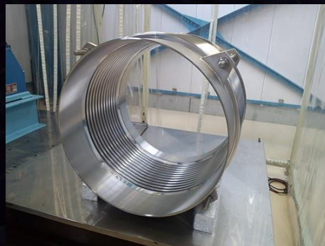
Bellows for each duct
