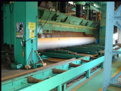
Press to form a duct
