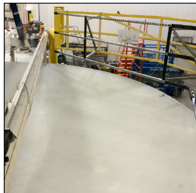
TAO 6.5-m mirror with front surface generated with 100 mesh metal bond cup wheel.
