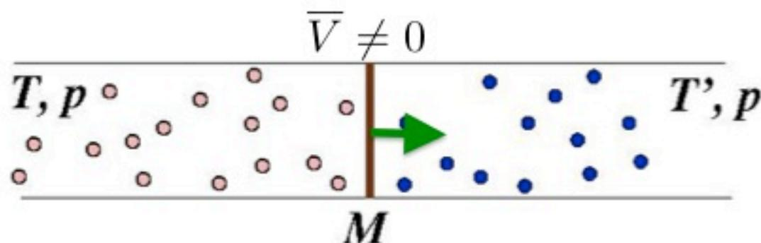
(i) Force on trapped adiabatic piston balanced by "spring"
