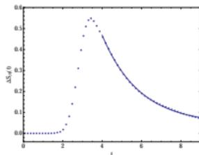
We see an initial time delay, rapid rise to the peak and decay. The best fit for the numerical results is exponential decay, with parameters depending on quench details.
