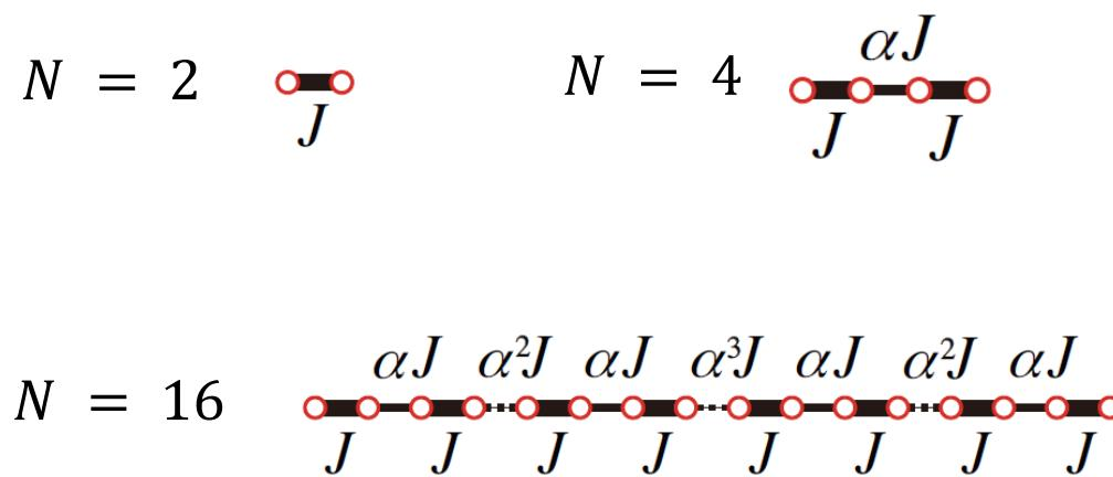
Connect two  $2^n$ -site units via exchange  $\alpha^n J$  to form  $2^{n+1}$ -site unit.
