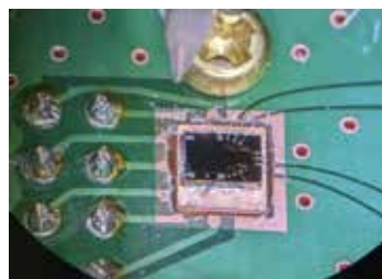
Fig. 1 A typical semiconductor device for quantum universe experiment and printed circuit board for the refrigerator.
