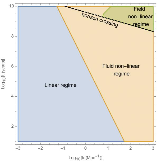
Approximate linear and nonlinear regimes in k-t plane for coupled DBI model with A=30. The dotted line shows horizon crossing: Fluid nonlinear regime starts when  $3/2 k^2 \Phi a_0^{-2} t_0^{4/3} t^{2/3} > 1$
