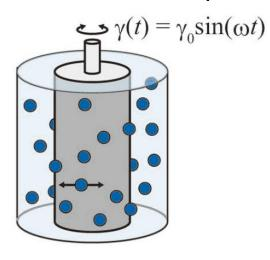
small  $\gamma_0$ : particles motion reversible large  $\gamma_0$ : particles motion irreversible
