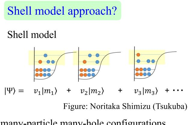
many-particle many-hole configurations in a mean-field potential →mixing by residual interactions
