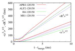
FIG. 11 (color online).  $\bar{R} (= \langle R^2 \rangle^{1/2})$  and  $\bar{Z} (= \langle z^2 \rangle^{1/2})$  as functions of time for APR4-120150, ALF2-120150, H4-120150, and MS1-120150.
