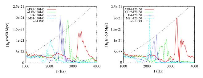
FIG. 10 (color online). Fourier spectra of gravitational waves for the results shown in Fig. 9. The amplitude is shown for the hypothetical event at a distance of 50 Mpc along the direction perpendicular to the orbital plane (the most optimistic direction). The black dot-dot curve is the noise spectrum of the advanced LIGO with an optimistic configuration for the detection of high-frequency gravitational waves (see https://dcc.ligo.org/cgi-bin/DocDB/ShowDocument?docid=2974).
