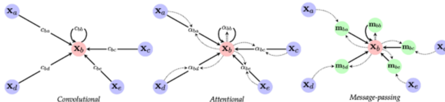
Figure 17: A visualisation of the dataflow for the three flavours of GNN layers, g . We use the neighbourhood of node b from Figure 10 to illustrate this. Left-to-right: convolutional , where sender node features are multiplied with a constant, c_{uv} ; attentional , where this multiplier is implicitly computed via an attention mechanism of the receiver over the sender: \alpha_{uv} = a(\mathbf{x}_u, \mathbf{x}_v) ; and message-passing , where vector-based messages are computed based on both the sender and receiver: \mathbf{m}_{uv} = \psi(\mathbf{x}_u, \mathbf{x}_v) .
