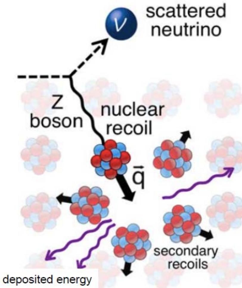
→ **WIMP dark matter detectors** developed over the last ~decade are sensitive to ~ keV to 10's of keV recoils
